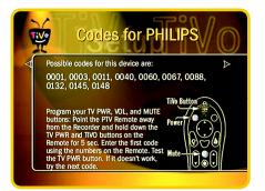
If you have your stereo hooked up to your TV, you can program the PTV Remote Control's volume and mute buttons to send signals to your stereo rather than to your TV. Go to Messages & Setup, then PTV Remote Setup, then PTV Remote - TV. Press the TiVo and VOL buttons to illuminate the LED before you enter the code.
